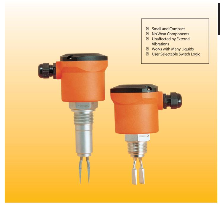
KOBOLD's NWS level switch works on the vibrating tuning-fork principle. A piezoelectric crystal is matched to the frequency of a tuning fork in air, and used to set the fork vibrating. When the fork becomes immersed in a liquid, its resonant frequency changes. The piezoelectric crystal is then no longer matched to the tuning fork. This causes the vibration to stop. The NWS's internal electronics detects this change and signals an alarm condition.
